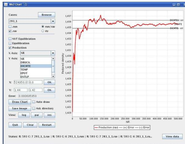
Figure 11: Snapshot of the tool *ms2chart*. The picture shows the analysis of a simulation of liquid cyclohexane.
