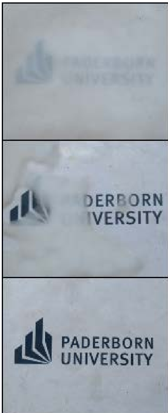
Fig. 4 Transparency of the present polymer compound from solid (up) to liquid (down).
