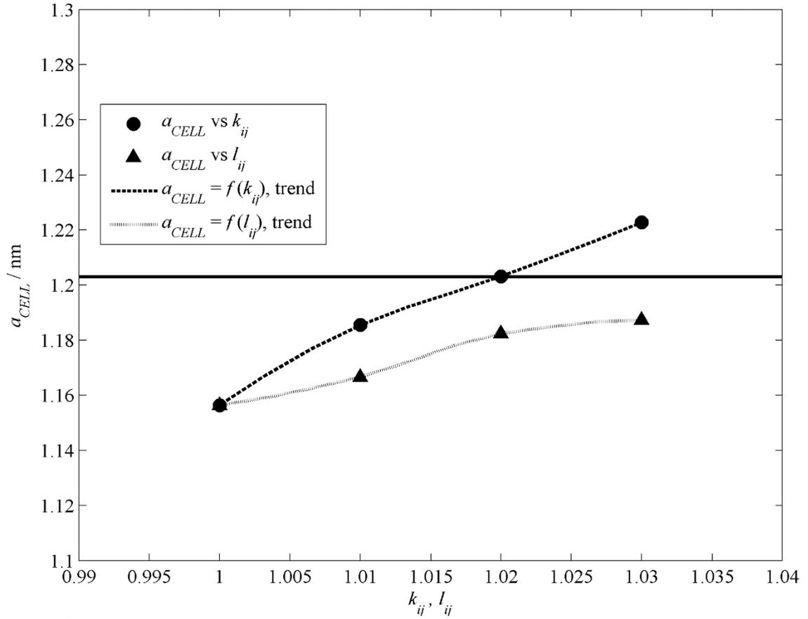
**Figure 5.** Effect of  $k_{ij}$  and  $l_{ij}$  on  $a_{CELL}$ . The solid horizontal line is the experimental value of  $a_{CELL}$  (1.203 nm) [15]. The trends are fitted as guides for the eye.
