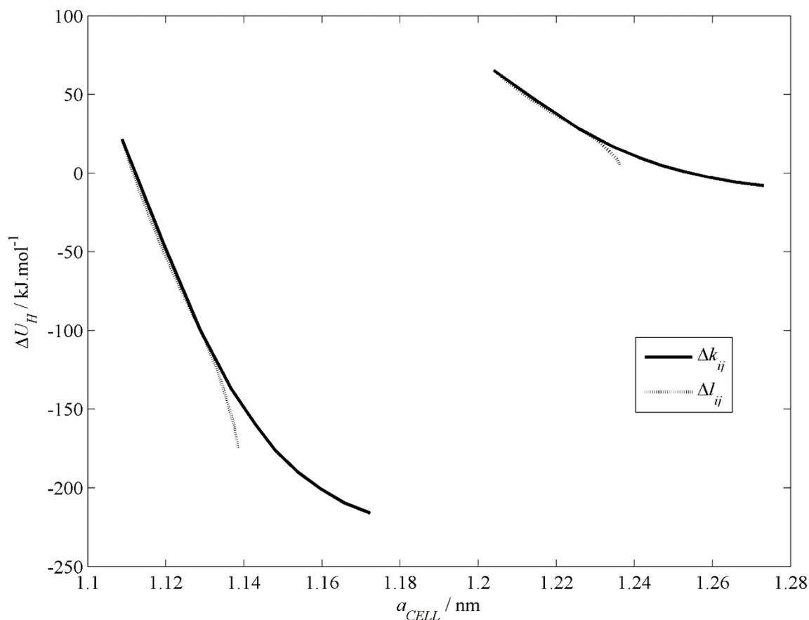
**Figure 9.** Estimates of allowed limits of  $\Delta U_H$  and  $a_{CELL}$  determined by separately changing  $k_{ij}$  and  $l_{ij}$ .
