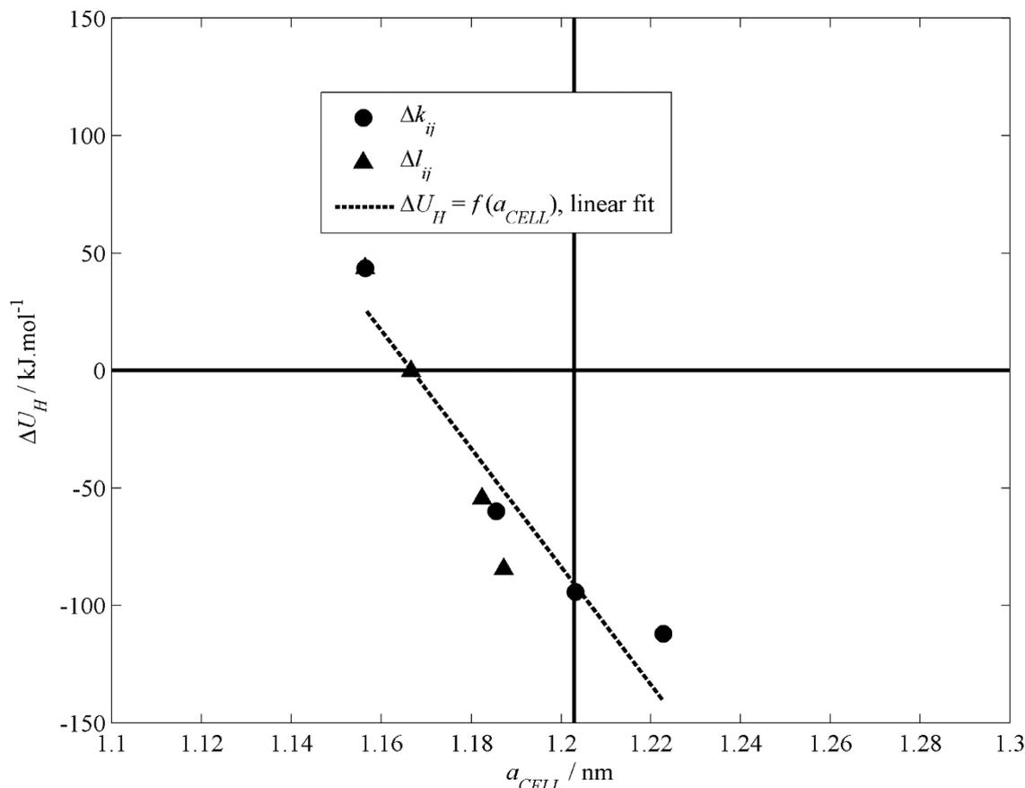
**Figure 6.** General trends for  $\Delta U_H$  vs.  $a_{CELL}$  determined by separately changing  $k_{ij}$  and  $l_{ij}$ . The horizontal solid line represents the value of  $\Delta U_H$  determined from experimental phase equilibrium data ( $\approx 20 \text{ J mol}^{-1}$ ), and the vertical solid line represents the experimental lattice constant (1.203 nm) [15]. The dashed line is a linear trend fitted as a guide for the eye.
