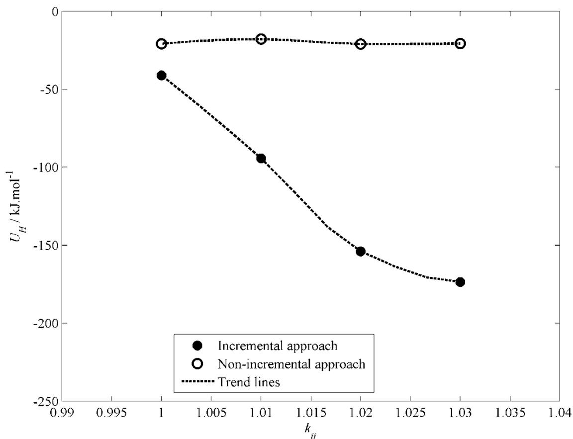
**Figure 1. Comparison of lattice energies of the empty sI methane clathrate hydrate calculated using incremental and non-incremental approaches in  $k_{ij}$ .**
