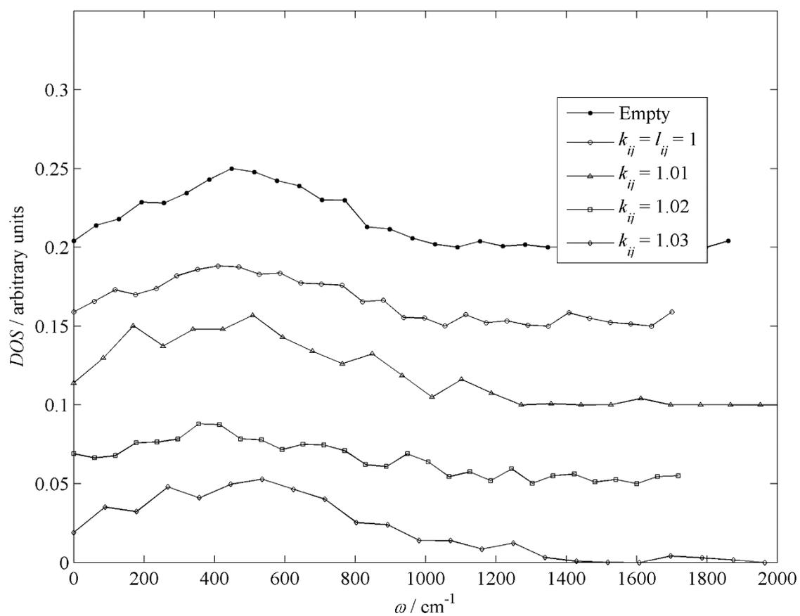
**Figure 2.** Influence of LJ dispersion correction factor ( $k_{ij}$ ) on phonon DOS of sI methane clathrate hydrate over the vibrational frequency ( $\omega$ ). Each plot is shifted upward from the curve below by 0.05 units for clarity.
