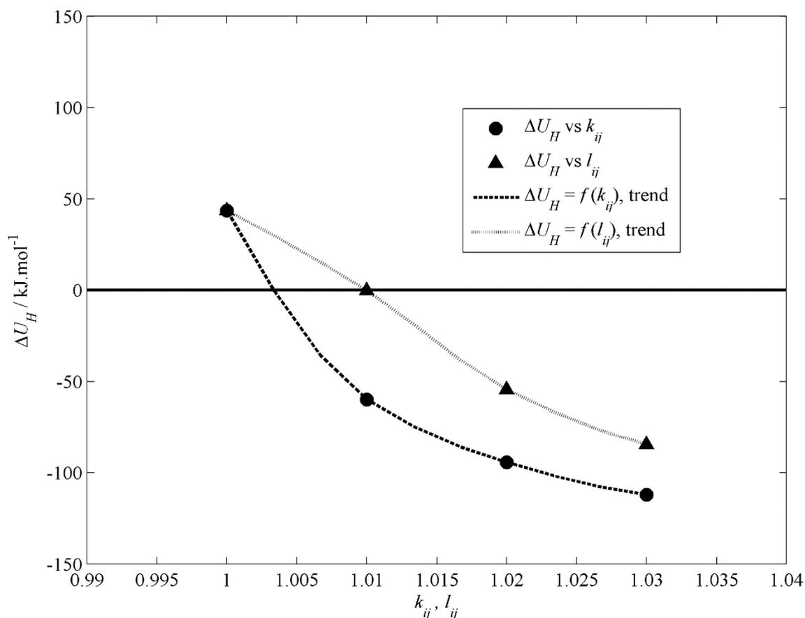
**Figure 4.** Effect of  $k_{ij}$  and  $l_{ij}$  on  $\Delta U_H$ . The solid horizontal line is the value of  $\Delta U_H$  calculated from experimental phase equilibrium data ( $\approx 20 \text{ J mol}^{-1}$ ). The trends are fitted as guides for the eye.
