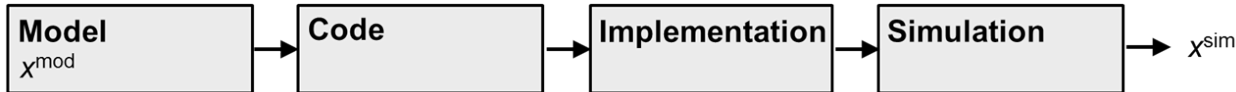
Figure 1: Schematic for the route from model to simulation result. The property x^{\text{mod}} described by the model is of interest and to obtain information on it, simulations have to be carried out. x^{\text{mod}} is not directly accessible, only the simulation result x^{\text{sim}} is. Errors may occur in every step of the route.
