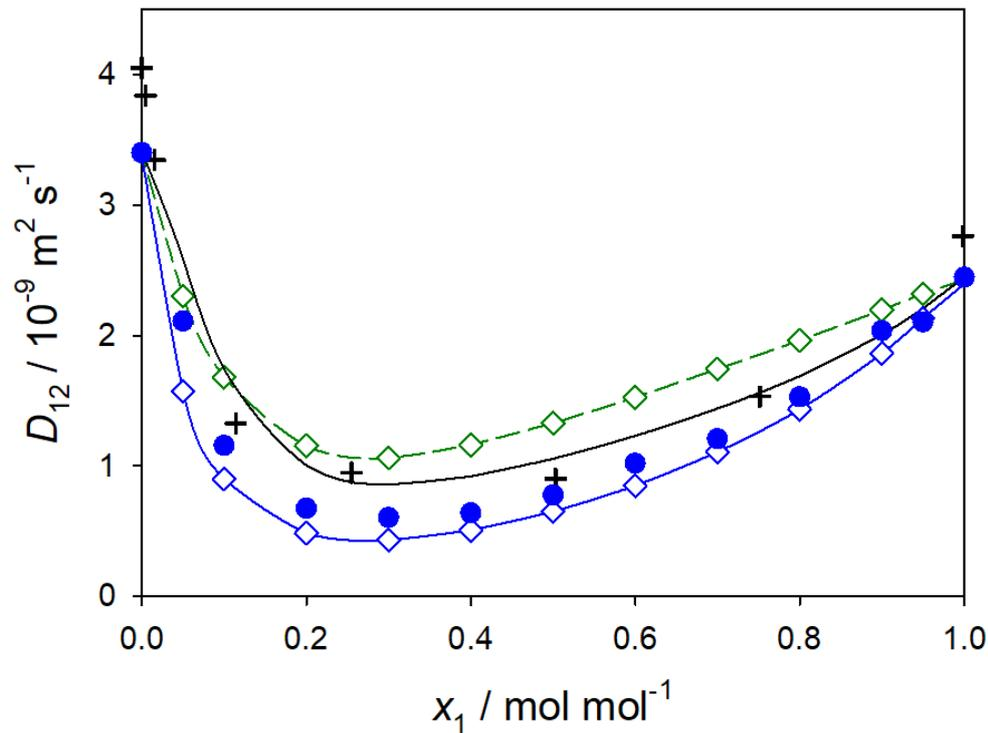
Fig. 2: Fick diffusion coefficient of the binary mixture methanol (1) + benzene at 298.15 K and 0.1 MPa. Simulation results (solid bullets) are compared with experimental data (crosses). The models by Li et al. (blue diamonds) and Zhou et al. (green diamonds) based on present simulation data are also shown.
