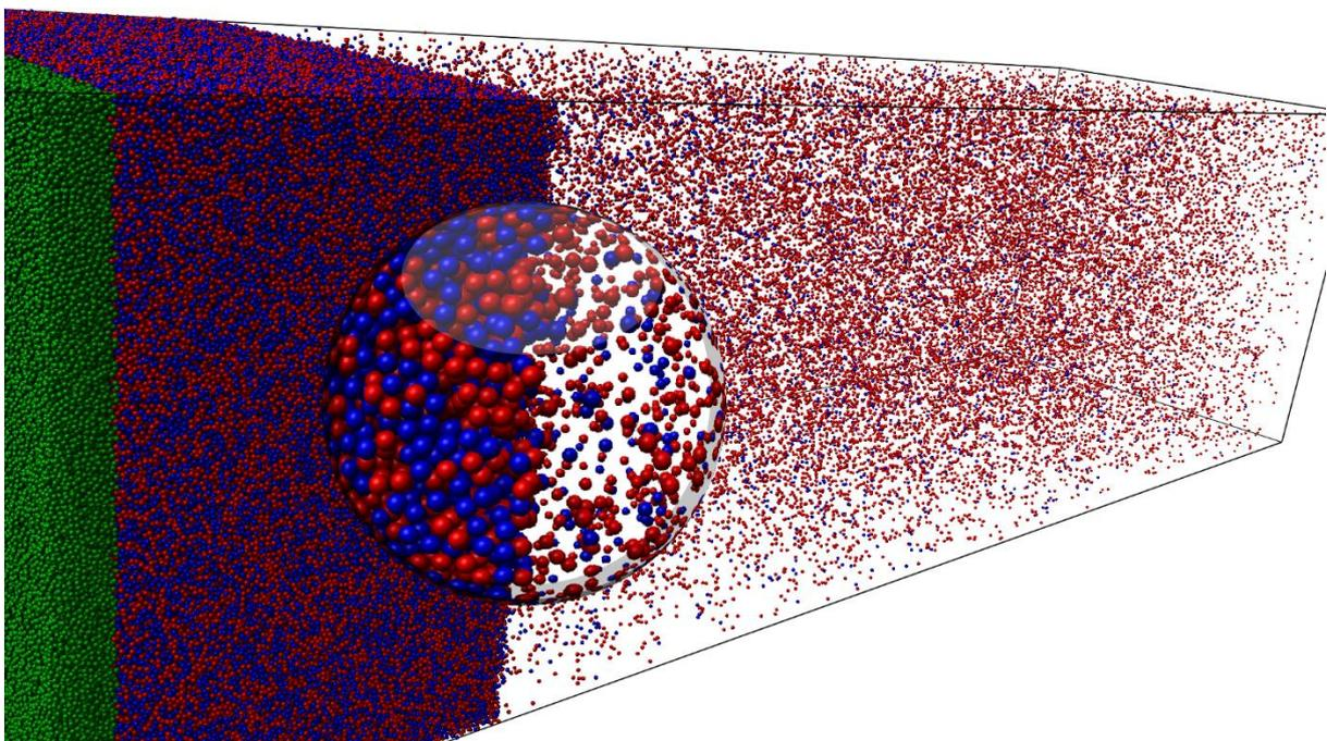
Fig. 1: Snapshot of a stationary simulation of evaporation into vacuum. The system consisted of a liquid and a vapor phase, connected through a planar interface. To the left, the liquid was extended by a reservoir, deployed for replenishment and thereby to attain stationary conditions. Particles constituting the reservoir, forward and backward particle flux are colored green, red and blue, respectively. The magnifying glass was added to support the visualization of the vapor-liquid interface.
